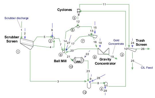
Figure 5 - Comminution Circuit Simulated in USIM PAC
