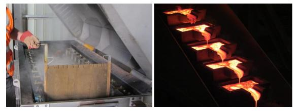
Figure 9 - First Gold Recovered at the Electrolysis Cells
