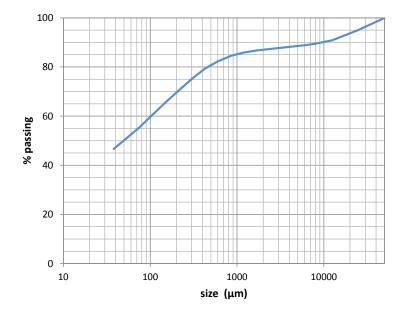
Figure 4 - Typical Particle Size Distribution of the Nampala Concentrator Feed
