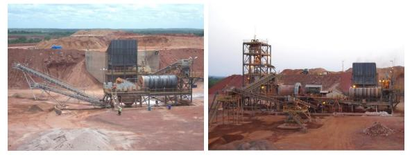
Figure 3 - Comminution Circuit - Before and After Phase 2 Expansion
